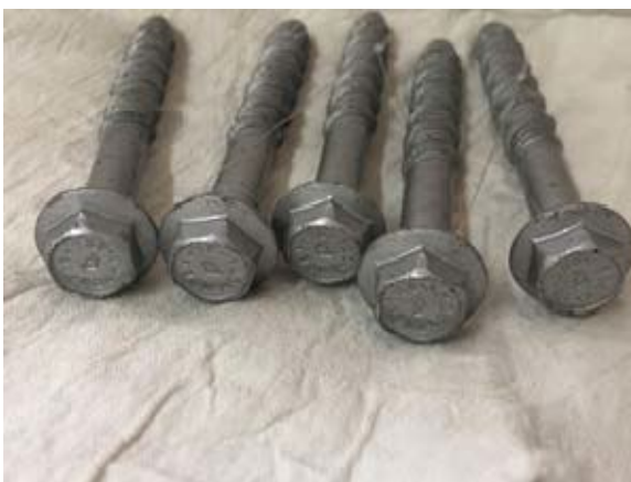
After testing 1008 hours
