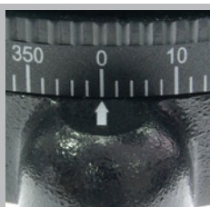
Freely rotatable horizontal circle
